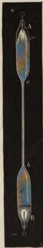
FIG. 73.—Geissler's tube, showing electric discharge.
